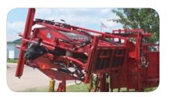
Lay-over feature offers up to 90° of rotation and offers a built-in, dropdown floor for increased convenience.
