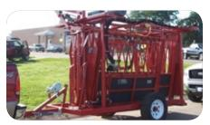
Portable Attachment balanced for easy positioning, the 2" x 4" steel frame with hand operated winch allows for one-man transport.
